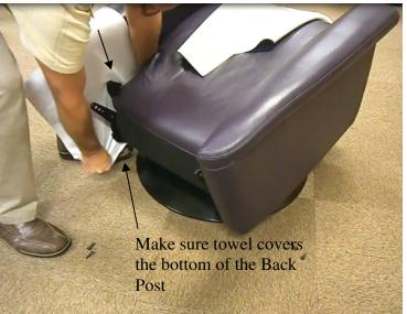
5. Slide a Towel between the Arm and the Back Post of the Mechanism all the way to the bottom as shown.
