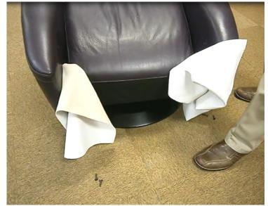
6. Towels shown on both Back Posts. The Towels will protect the Inside Arm Leather from scratches.
