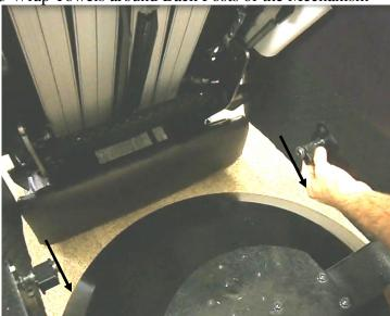
5. Tilt Seat Assembly down until the Tracks line up with the Shoes – Long portion of the Shoe should face the rear of the Chair as shown
