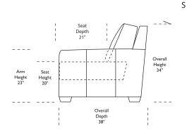
\*Note: arm height for this frame is measured at the highest point of the arm.
