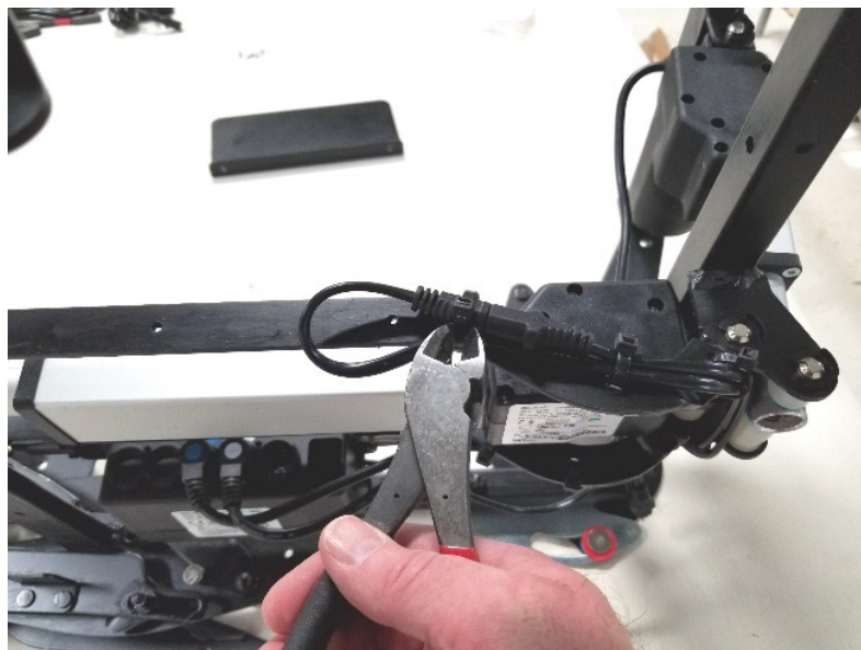
Cut Zip Tie from Power Extension Cords as shown
