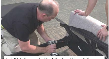
Install 2 Bolts on each side of the Camel Hump Rail
